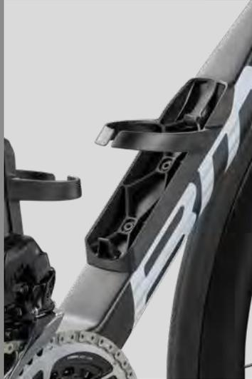
Every design element on the Teammachine R was conceived as a complete package – even the bottle cages. The ultralight carbon bottle cages on the Teammachine R keep the bottles low and shielded from turbulent air which helps lower the center of gravity and actually makes the bike faster with bottles onboard.
