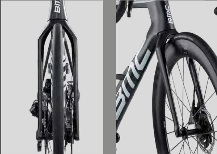
The ultrawide parallel fork legs are unlike anything else in the peloton. When rotating at speed, the front wheel produces a significant amount of turbulent air. We increased the inner fork spacing to allow that turbulent air to be shuttered away from the frame and reduce aero stall. The result is cleaner air that hugs the frame longer resulting in a significant drag reduction.
