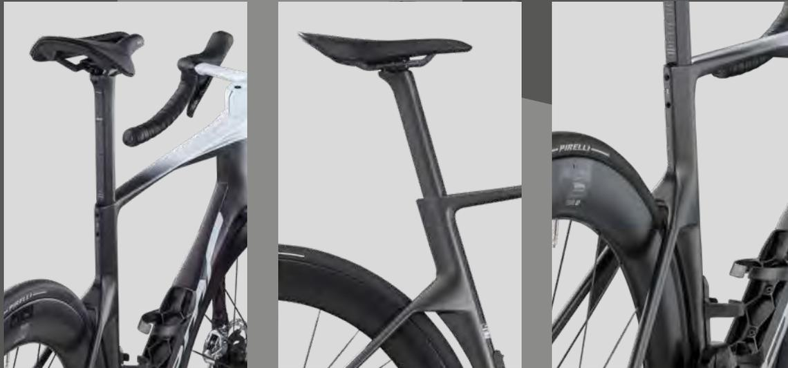
The new Teammachine R seatpost isn't just slimmer, deeper, and more compliant - keeping the aerodynamics optimized with a redesigned shape that reduces frontal exposure without a loss in comfort or ride characteristics.
