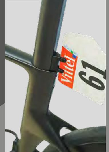
In the creation of the Teammachine R, no detail was overlooked, no matter how small. An example of this is the purpose-built Race Number holder. Seamlessly integrated into the seatpost, this design innovation eliminates the need for glue or zip ties, reflecting our commitment to both aesthetics, functionality and of course, racing.
