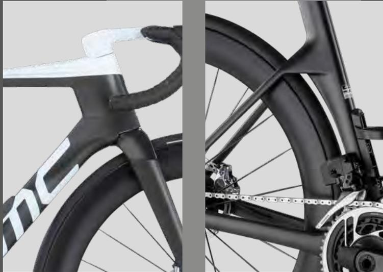
We knew pushing the envelope of the updated UCI limits on frame shapes could be tricky, but it was a challenge we ran to, rather than from. Again, borrowing lessons we learned from the Speedmachine, we expanded the horizontal profile in key locations like the head tube, bottom bracket, and seatstay junction. The resulting shapes not only look fast but enable the Teammachine R to respond more effectively across a wider range of yaw angles.
