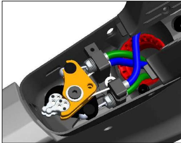
**In green the standard** routing from the brake booster to the brake caliper.
