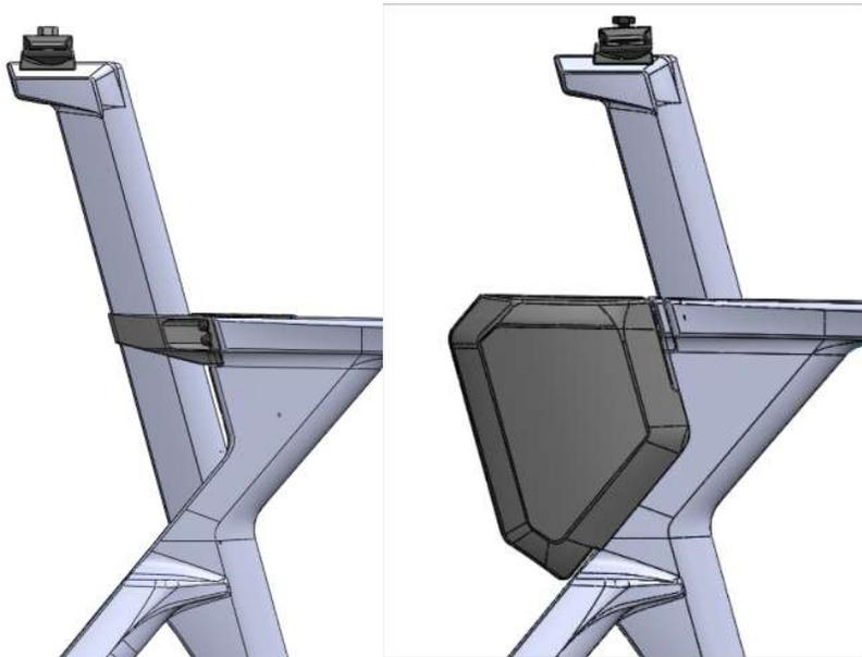
The forward mounting option enables the use of a storage box.
