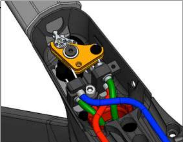
The distance from end of casing to brake stoppers have to be **32mm (see page 46)**.
