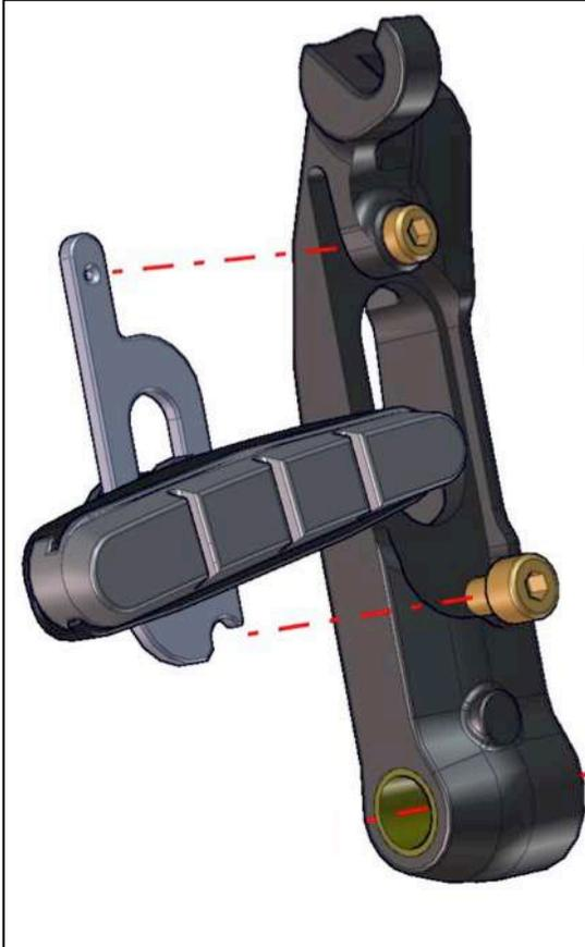
The Quick Pad feature (patent pending) is an easily removable brake pad cartridge system available only on Timemachine 01.
