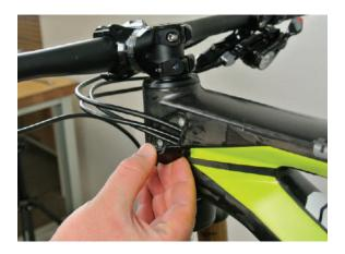
When replacing cable housings we recommend leaving the cables in place so they can guide the new housing.
