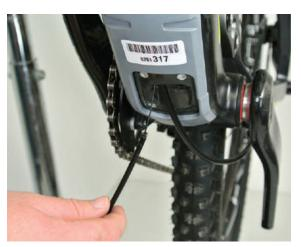
Pull the cable housing out of the frame towards the bottom bracket.
